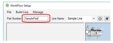
Click the Processes to build the Parts' Process Flow.
